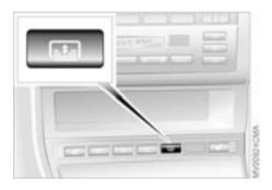
To actuate, press the button briefly with the ignition key in position 1 or higher.
